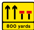
Temporary lane closure (the number and position of arrows and red bars may be varied according to lanes open and closed)
