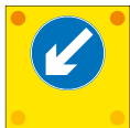
Slow-moving or stationary works vehicle blocking a traffic lane. Pass in the direction shown by the arrow.
