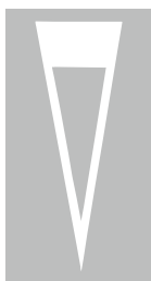
Warning of 'Give Way' just ahead
