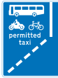
With-flow bus lane ahead which pedal cycles, motorcycles and taxis may also use
